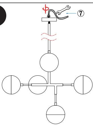
7.Take out the screw on the tube, insert the ceiling canopy into the wire, and then install the screw and gasket, tighten and fix.
