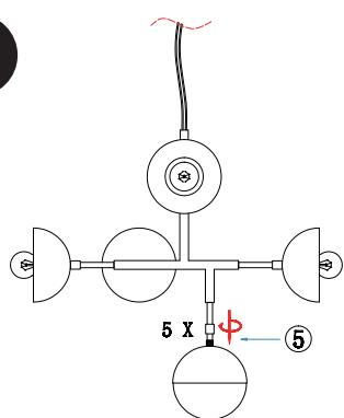
5.Complete the installation of the glass lampshade, put down the metal lampshade and the glass ball completely fit, and screw down the nut to fix the whole lampshade. Follow steps 2-5 to complete the assembly of all 5 glass lampshades
