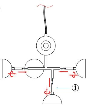
1. Take out the whole lamp from the carton, then push one of the lamp holder tube towards the direction of the lamp body according to the picture, plug the connecting wire into the corresponding screw thread tube at the same time. Finally, screw the two tubes tightly into each other. Tighten the 5 light tubes according to this step.
