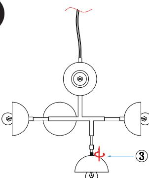
3. Unscrew the nut at the top of the metal lampshade
