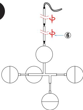
6.Take 2pcs L:500mm X Dia.11.5mm tubes and connect them to the lamp body through the top wire. Tighten and fix the lamp tube
