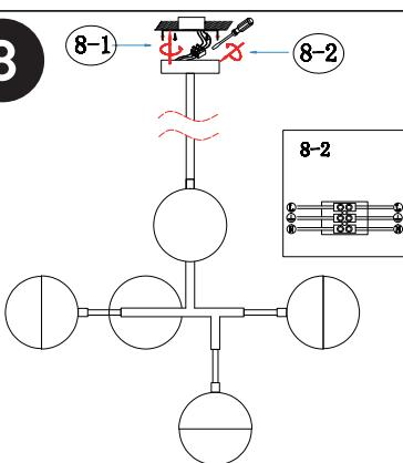
8.Switch off the mains supply; Drill 2 holes on the ceiling where the fixture is located; Put the expansion plug in hole and the silver metal hanging bracket on the ceiling; Connect the wire to the white terminal, connect the wire to the ceiling.
