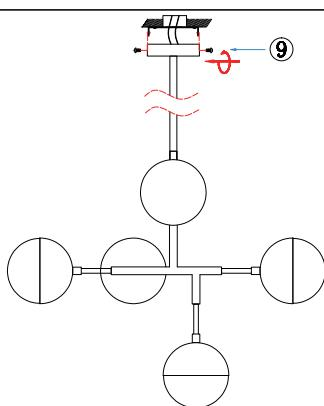
9.Fix the whole lamp and the ceiling canopy on the hanging bracket, and tighten the screws to complete the installation.
