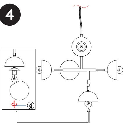
4.Lift up the metal lampshade, take a glass lampshade and wrap it around the white plastic sheets. Glass lampshade needs inclined angle, put into from the break of white plastic sheets, it can install glass lampshade completely on lampholder after rotating one circle
